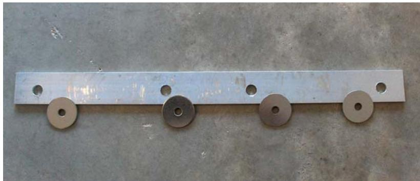
Step 9: Install grab rail & stainless steel backing plate; the lip on the bottom of the plate faces the boat. Fill holes (front/back) w/silicon before/after pushing bolts all the way through. Install support bracket, add 4 washers and 4 nylon lock nuts (1/2" ratchet wrench).
