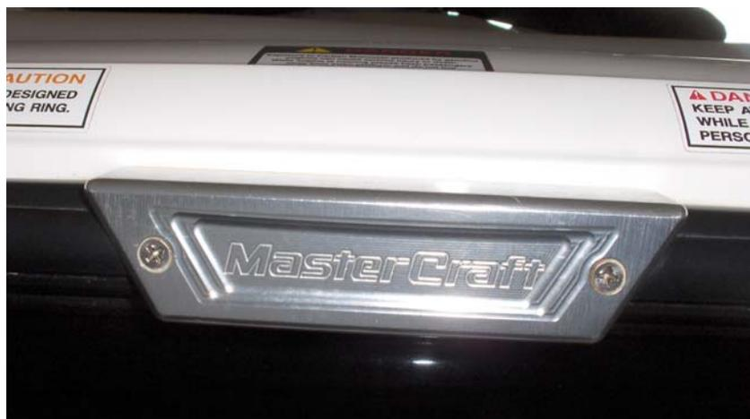
Step 2: Place a pencil mark on the boat where the two rub rail ends meet to use later as one reference point for centering the grab rail.
