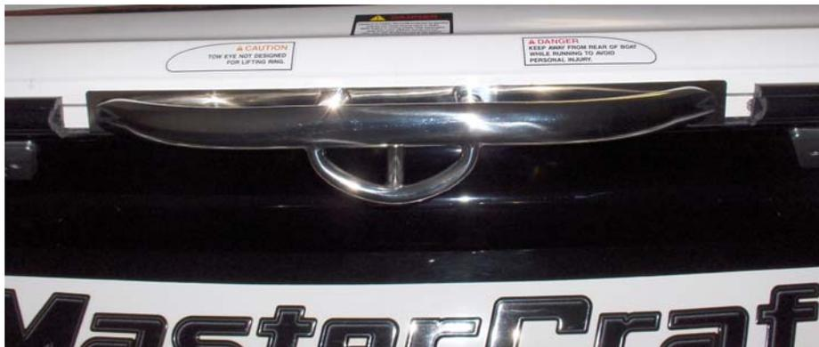
Step 11: Reinstall rub rail. Use hairdryer to help soften the material and a large flat blade screw driver to push it back into the rail.
