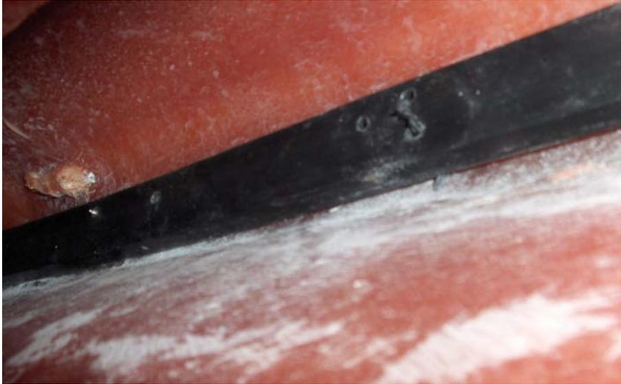
Step 8: Drill 4 holes in the boat and 4 holes in support bracket. To prevent chipping the fiberglass, use smallest drill bit first and then worked up to a 5/16" bit.
