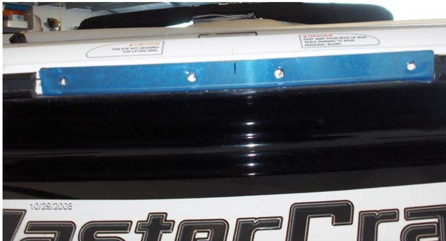
Step 7: Remove flooring/backing from storage area to ensure no wires, etc are in the way. The rub rail is anchored by a 1" x 1/4" plastic composite strip.
